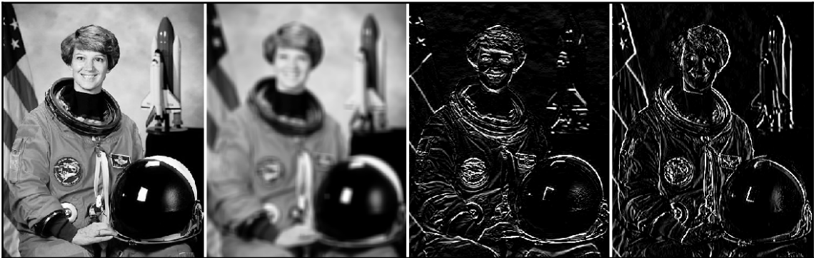
The first image is the grayscale input. The second image is the result of a 10 x 10 blur filter. The third and fourth images use detectors and vertical Sobel edge detector
