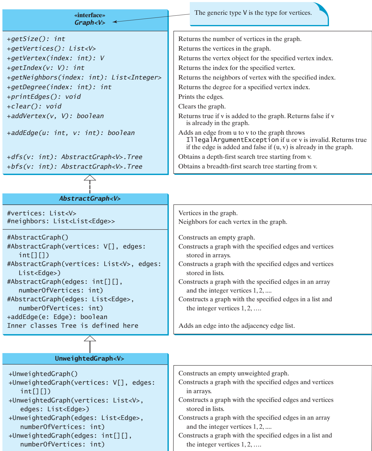
FIGURE 28.9 The Graph interface defines the common operations for all types of graphs.
