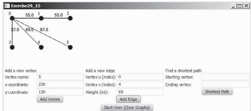
FIGURE 29.27 The program can add vertices and edges and display a shortest path between two specified vertices.
