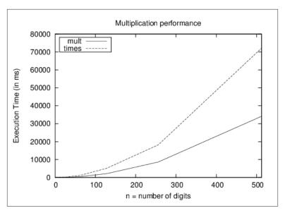
Figure 2-4. Comparison of mult versus times
