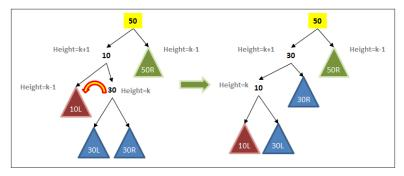
Figure 5-12. Rebalancing the Left-Right scenario
