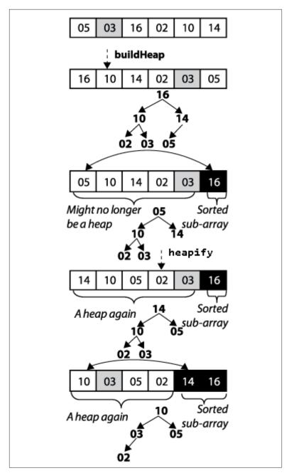
Figure 4-4. Heap Sort example
