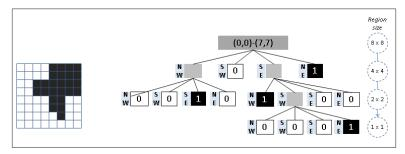
Figure 10-3. Quadtree using Region-based partitioning
