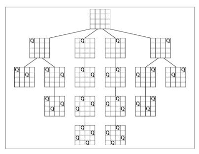
Figure 11-3. Final solution for 4-Queens Problem with four rows extended
