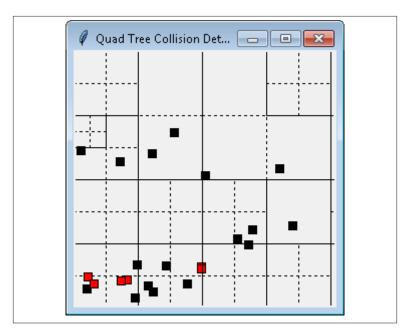
Figure 10-14. Collision detection using a quadtree
