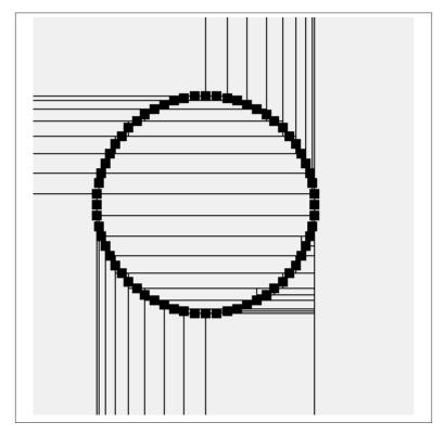
Figure 10-8. Circular data set leads to inefficient kd-tree
