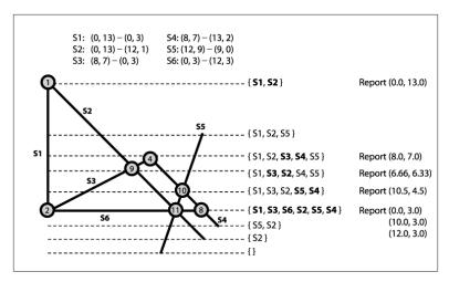
Figure 9-7. Detecting seven intersections for six line segments
