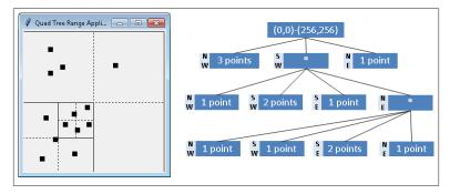
Figure 10-4. Quadtree using Point-based partitioning
