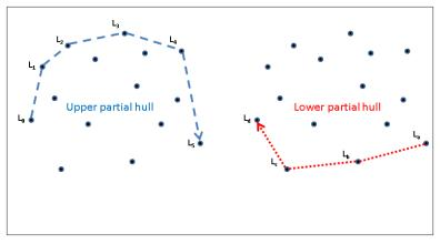
Figure 1-4. Hull formed by merging upper and lower partial hulls
