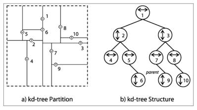
Figure 10-2. Division of two-dimensional plane using kd-tree
