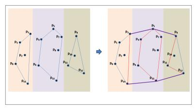
Figure 1-5. Hull formed by parallel constructions and stitching
