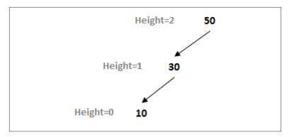
Figure 5-8. Unbalanced AVL tree
