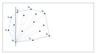
Figure 1-3. Hull formed using greedy approach
