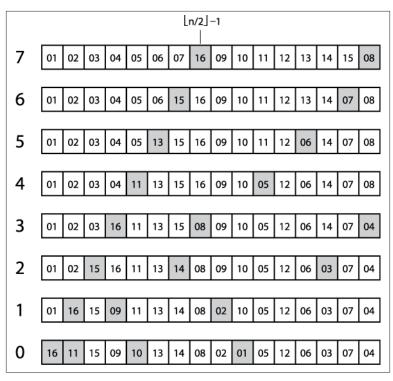
Figure 4-6. buildHeap operating on an initially sorted array
