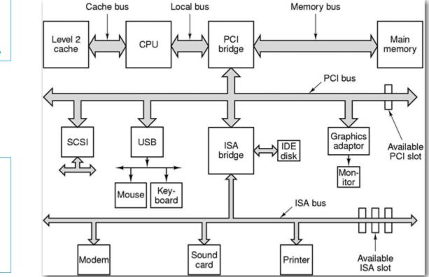
Any of these devices can cause an electrical interrupt that grabs the attention of the CPU.
